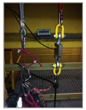
Test of back-up tools for rope access on loaded ropes, 13th of december, 2012.  $\ensuremath{\mathbb C}$  BARA. Page 4.
