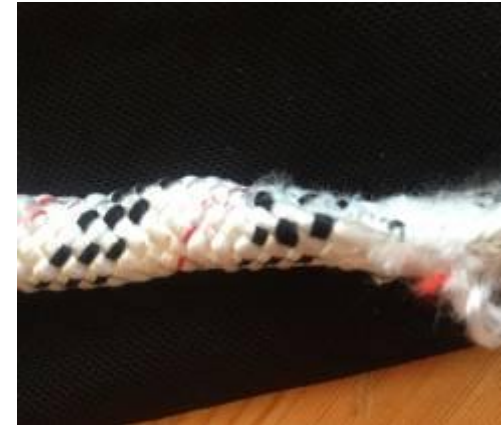
1 st 100kg Drop Test - Lower end - of failed sheath showing crushing at the point that the ASAP 'locked on'. The taper is where the wheel stopped and the shape is permanent due to heat distortion.
