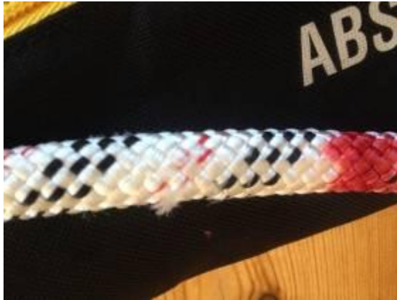
2 nd 100kg Drop Test. Minor damage to rope caused by teeth. Red mark indicates stopping position of the top edge of the ASAP. The damage is where the teeth locked on.
