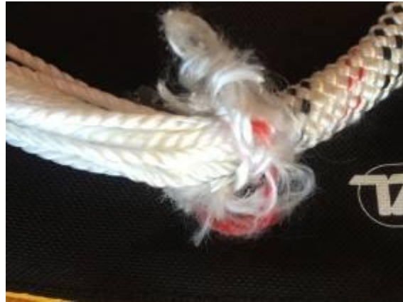
1 st 100kg Drop Test - Top end - Sheath failure and two of core strands, this is at the same position as on 2 nd test.
