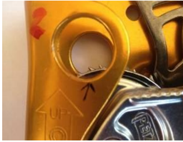
Damage after 100gk Drop test – section of 'wheel' visible
