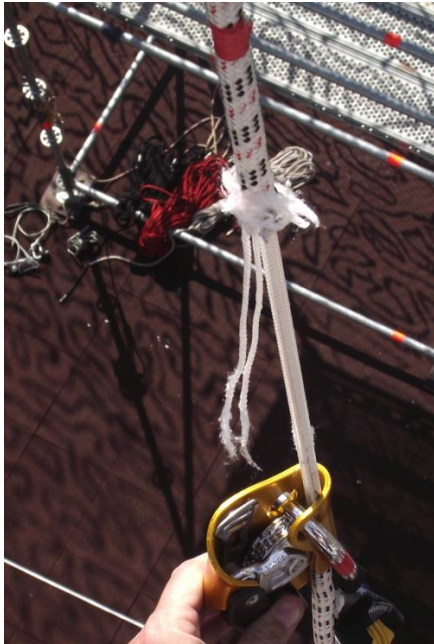
Damage – 1 st ASAP 100kg Drop Test
