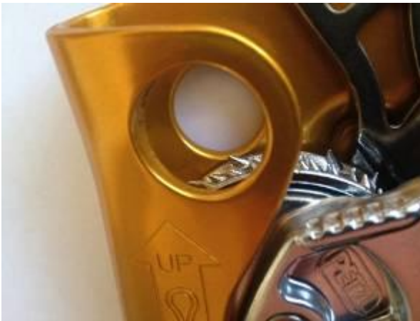
New – No damage to body at clip point.
