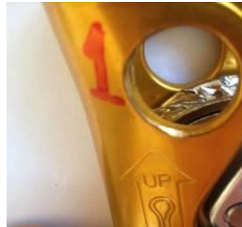
Deformation caused by Karabiner during 100kg drop test.
