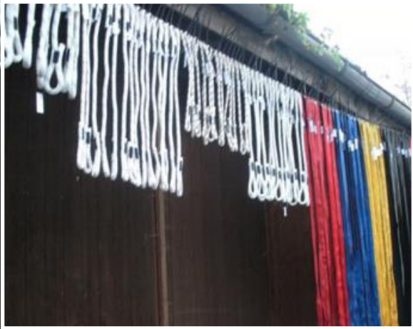
Since 2010 continuously aged testing samples for long time performance investigation and proof
