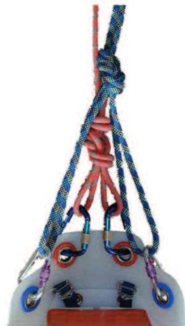
Fig 2 Alternative Vertical Lifeline Attachment When using this method all of the haul points must be used to ensure that the load is shared.
