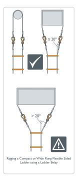
A Ladder Spreader may be used to achieve the correct angle where a Compact Flexible Sided Ladder is rigged from a single anchor point. Never join the ends of a ladder together unless the ladder has been made with long 'tail ends' or a single eyelet at the top (LV).
