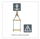
Note I: Compact Flexible Sided Ladders with code LV are designed to be fixed to a single anchor point.
