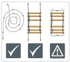
When securing a rolled up Flexible Sided Ladder, do not distort the ends of the side wires.
