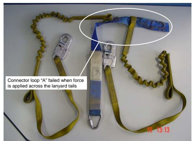
Figure 2 – Failure of lanyard at loop "A"
