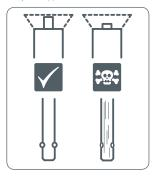
Figure shows left pin in good working condition. The right pin should be retired due to wear and detent pins not properly working.
