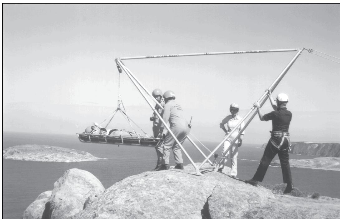
ground feet can be fitted and a star picket driven through the triangular hole. If for any reason the hinge spike cannot be used the Larkin Rescue Frame is still very stable and any slippage of the
