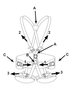
Step into harness, fasten and adjust in the order 1 - 2 - 3 in the diagram. If necessary the rear D-ring may be adjusted up and down by sliding the webbing through the buckle arrangement.
