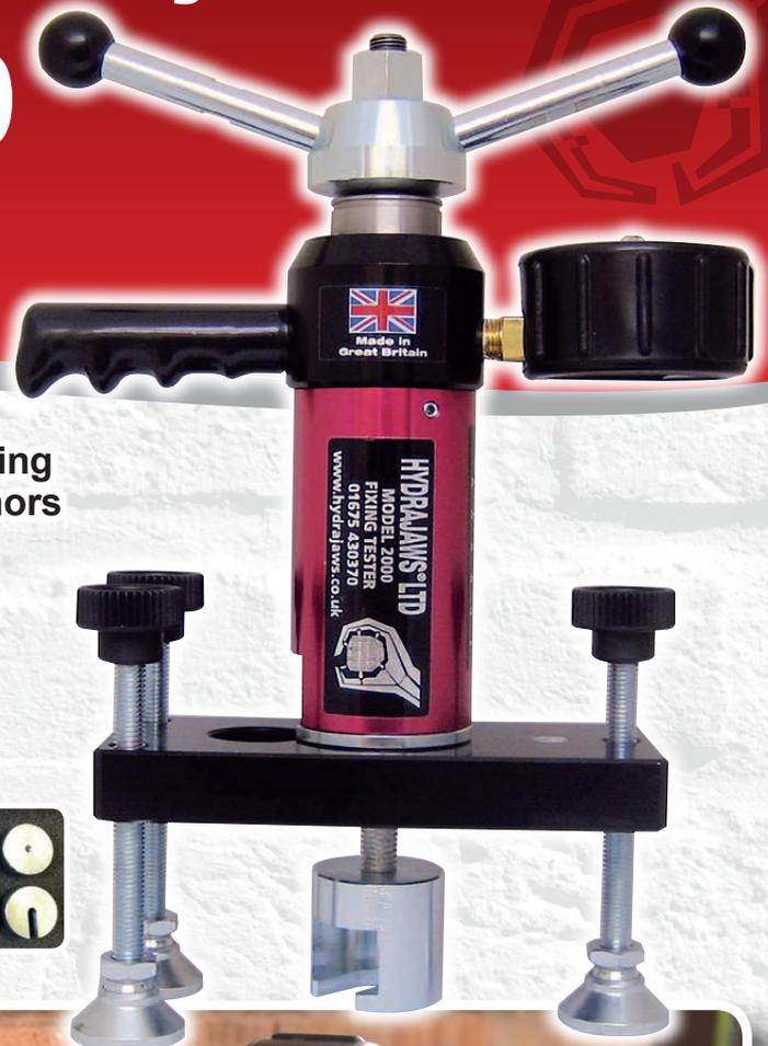
**Model 2000 Medium Duty Fixing Testers - enabling engineers to confirm the holding power of anchors in most construction materials.**
