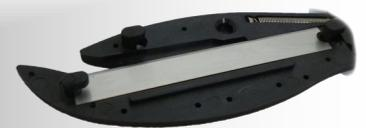
Remove locking screw & slide the top half of the knife back until you can lift it off. Reverse or replace blade(s) with care. Replace top half of the knife & slide back into place. Replace locking screw.
